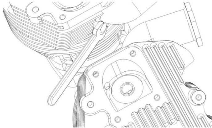
12. Single Carb Only: the Y-Split intake manifold needs to be attached to an engine after both heads are in place. Minute adjustment of the head positions (clocking) is recommended before final fastening the head bolts. Use the exposed openings of the manifold to “clock” the heads for best fit that provides small, uniform gaps between the manifold and both intake ports.
