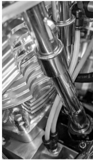
16. The exhaust outlet has been designed to fit either single-bolt OEM headers or the common, three-bolt aftermarket flanges. The exhaust port ID has been designed with a minimum clearance over the stock exhaust pipe stub – in some cases (e.g. deformed header) a careful grinding of the stub's OD may be required.
