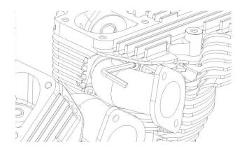
\*\*\*SHOVELHEAD head pictured for reference only\*\*\* For an easy access, Double (shown) and Single Intake Manifolds require SHCS bolts on the top (use ball-end Allen key) and HEX bolts on the bottom (use flat wrench).
