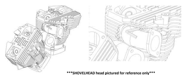
For an easy access, Double (shown) and Single Intake Manifolds require SHCS bolts on the top (use ball-end Allen key) and HEX bolts on the bottom (use flat wrench).
