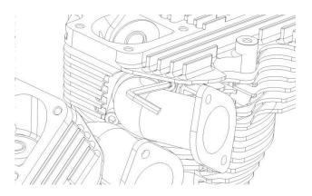
For an easy access, Double (shown) and Single Intake Manifolds require SHCS bolts on the top (use ball-end Allen key) and HEX bolts on the bottom (use flat wrench).
